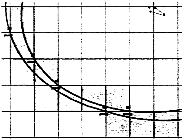
Figure 8.18. The \alpha\beta -infinite hull of a digital elliptical arc, where r_x = 6 and r_y = 4 . The domain of the digital arc is also shown.
