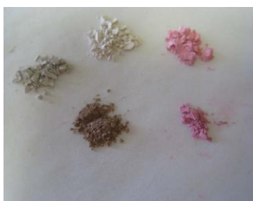
Figure 4.2 (A) Slurries of TiO 2 nanoparticles with left to right: TPP, (TPP)Zr(OAc) 2 , Zn(TPP) and (TPP)Hf(OAc) 2 . 30 mg of TiO 2 nanoparticles were treated with 2 ml of 0.5 mM porphyrin solution by mixing slurry overnight, removing the solvent, and rinsing 2-3 times with toluene. (B) Powders on upper row from left: TPP, Zn(TPP) and (TPP)Zr(OAc) 2 ; lower row from left: TCPP (THF used as solvent and for rinse) and (TPP)Hf(OAc) 2 .
