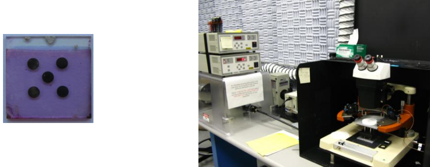
Figure 4.22 Image of five masked solar devices and Oriel 9600 150 W solar simulator with an AM1.5G filter used for photovoltaic measurements.
