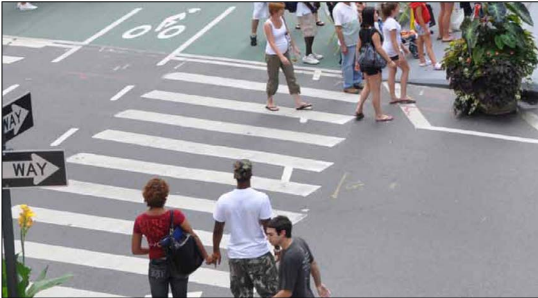
Figure 5.7 High Visibility Crosswalk in New York City (Source: New York City Department of Transportation 2010b, p. 19)
