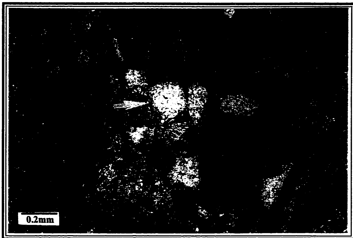
Figure 5-13. Lithofacies 8- Quartzose dolostone with anhydrite laths. Photomicrograph of a thin section under crossed nicols, showing anhydrite laths (arrow) that display bright second-order interference colors. Note the fine textured dolomite matrix.
