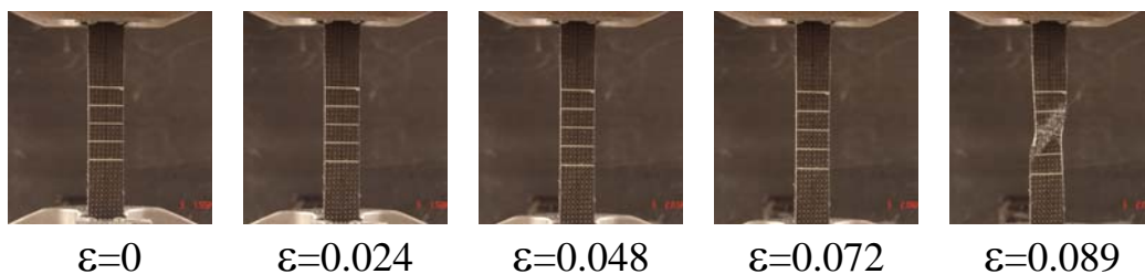
Figure 3.4 (b) Optical pictures of GR/GL/GR (+45/-45 fiber orientation) specimen taken during room temperature tensile testing at different strain levels.
