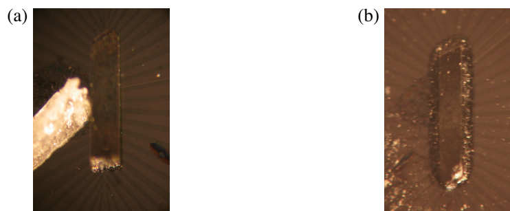
Figure 87: (a) The sample was normally directly mounted on the Hall-sensor chip (see Fig. 78). The white chunk in the left side of the picture is Eicosene (a kind of bee's wax), which melts at a temperature a little higher than room temperature. A small amount of it was applied next to the sample and was heated up by a light bulb for a short time until it was melted. (b) Once the Eicosene melts, it surrounds the sample and holds it fixed to the sensor.
