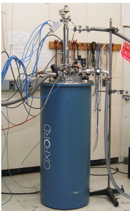
Figure 68: A commercial Oxford top-load ^3\text{He} cryostat was used to do most of the measurements. This side view photograph of the ^3\text{He} cryostat shows the system with the probe in the “down” position (see also Fig. 70).
