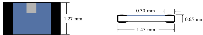
Figure 89: The dimensions for bare chip model of ruthenium oxide thermometer (RX-102A-BR by Lake Shore) are shown. The active surface (thick film) was directly mounted on the sample to measure the temperature as shown in Fig. 64.
