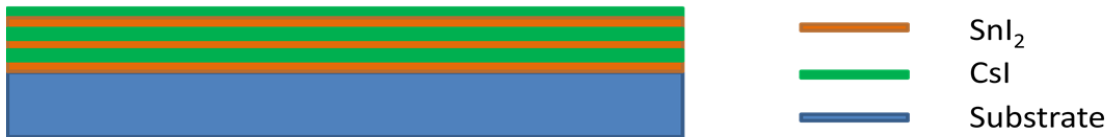
Figure 3.9: Schematic of CsSnI 3 precursor deposition procedure. SnI 2 and CsI are deposited alternately for 6 layers in total.
